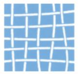
Wires in typical screen packs can shift under pressure resulting in reduced filtration. (not sintered)
