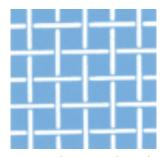
In sintered screen packs, each wire is permanently bonded in place at every contact point.
