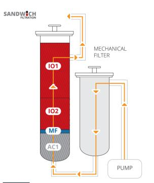
This system makes it possible to rinse PBCs or stencil with de-mineralised water with a conductivity of about 0.5 μS and a pressure of 0.2 bar.
